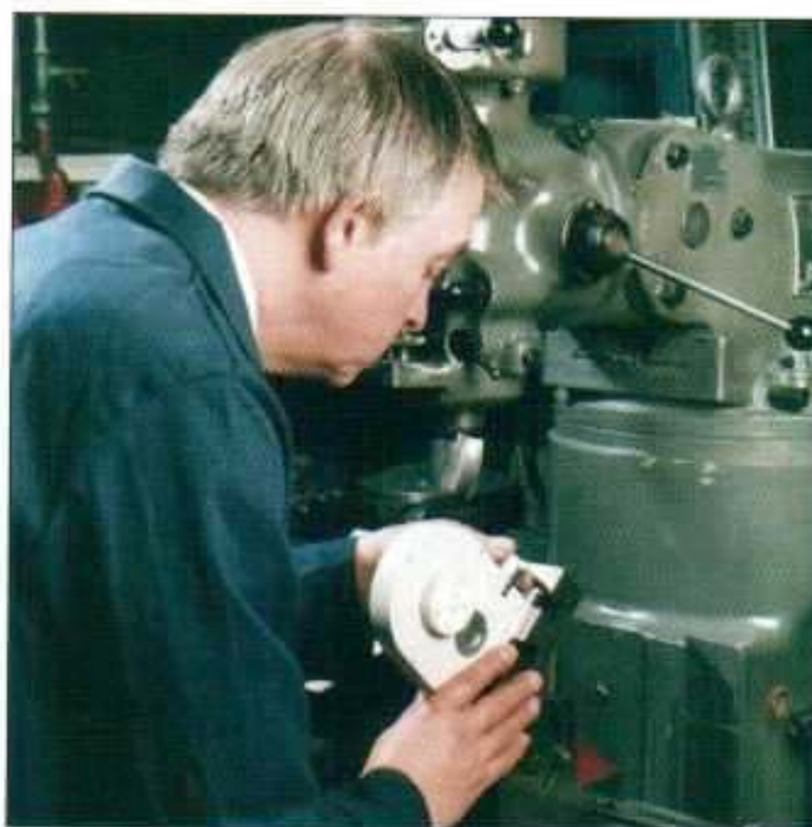
Checking workpiece angle using TB121 clinometer
